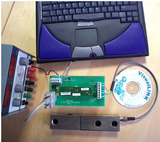
Figure 2.4 DSC2-RS232 Versions Evaluation Kit Connections
