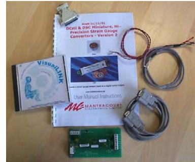
Evaluation Kit for the RS232 with the DSC
