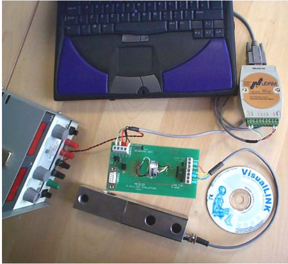
Figure 2.2 DCell - RS485 Versions Evaluation Kit Communications
