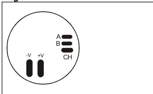
Figure 13.3 DCell Bus Connections
