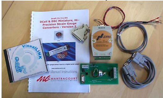
Evaluation Kit for the RS485, with the DCell
